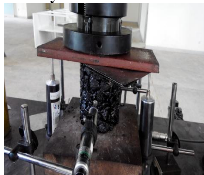
Figure 2. Tist Loads and Stress Asphalt by UTM Machine
